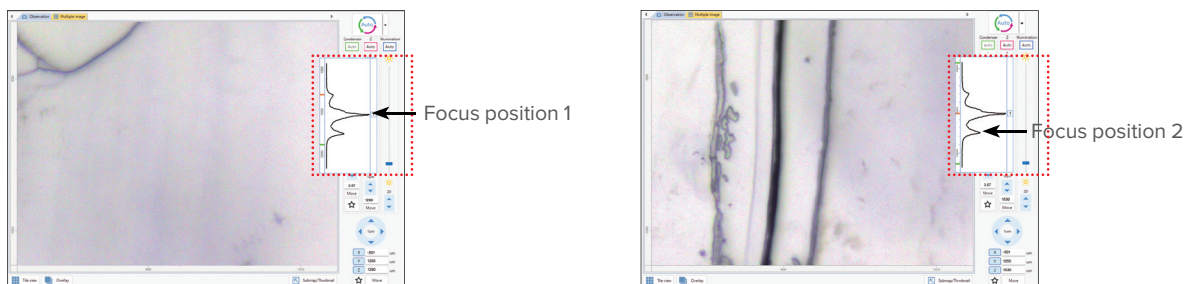
Observation image using x16 cassegrain mirror - KBr plate of multilayer film for food packaging -
